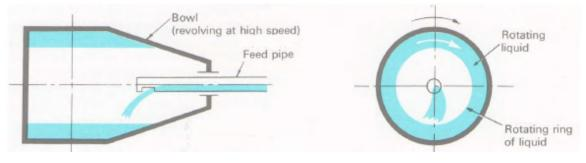
THE PRE-TREATENT LIQUID (SUSPENSION) IS FED VIA THE FEED PIPE INTO THE BOWL, WHICH IS REVOLVING AT HIGH SPEED.
