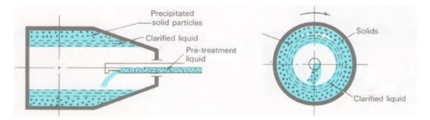
THE CENTRIFUGAL FORCE EXERTED ON THE LIQUID AS IT FORMS A REVOLVING RING INSIDE THE BOWL, IS ENORMOUS; AS MUCH AS 3500 TIMES THE FORCE OF GRAVITY (3500 X G). THIS MASSIVE CENTRIFUGAL FORCE CAUSES THE SOLID PARTICLES WITH A HIGH DENSITY PRESENT IN THE LIQUID TO QUICKLY PRECIPITATE, SO THAT TWO SEPARATE LAYERS, ONE OF SOLID PARTICLES AND ONE OF CLEARED LIQUID, ARE FORMED ON THE INNER WALL OF THE BOWL.
