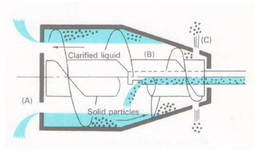
FOR THE DISCHARGE OF THE SEPARATED SOLID PARTICLES, THE SCREW CONVEYOR (B) TURNS AT A FRACTIONALLY DIFFERENT SPEED TO THE BOWL, THUS CONVEYING THE SOLID PARTICLES TOWARD THE CONICAL END OF THE BOWL, WHERE THEY ARE DISCHARGED BY CENTRIFUGAL FORCE THROUGH THE SOLIDS DISCHARGE OUTLET (C) LOCATED AT THE NARROW END OF THE BOWL.
